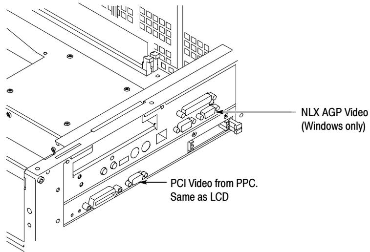
**Figure 6-37: PCI and NLX video connectors**
