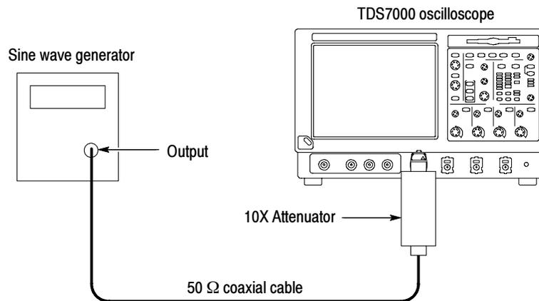
**Figure 4-25: Initial test hookup**
