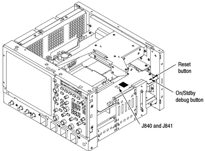
**Figure 6-38: Location of jumpers and reset button**
