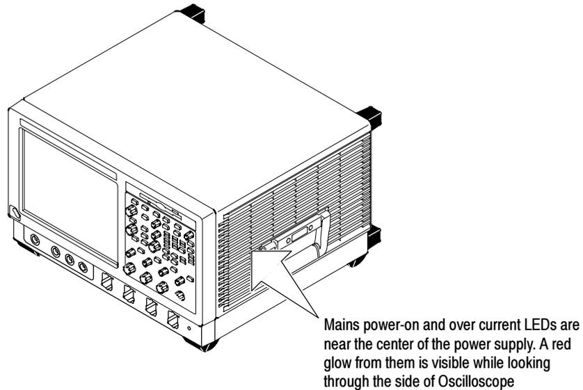
**Figure 6-33: Location of power-on and over current LEDs**
