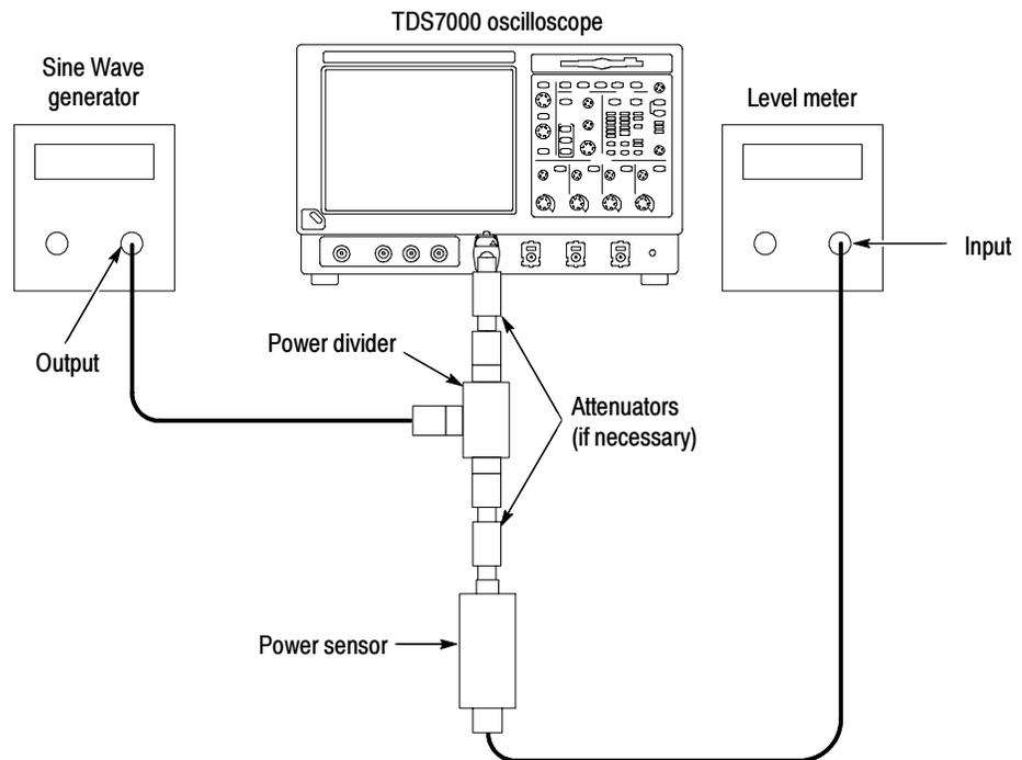
**Figure 4- 41: Sine wave generator leveling equipment setup**
